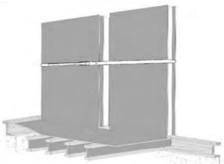
Set the splines into the grooves of the fixed (standing) panel. Bring your connecting panel into position over the bottom plate, tilted slightly away from the fixed panel. Butt the skins together at the bottom and scissor the walls together using a sharp motion.
