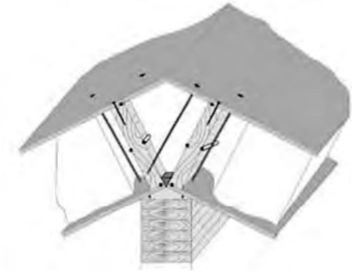
**Vapor Retarder** – An appropriate vapor retarder must be installed on the interior of the roof panels. Premier recommends using SIP tape on the panel joints and at the wall to roof connections. Refer to Technical Bulletin #28 at [www.premiersips.com](http://www.premiersips.com) for more information on this subject.
